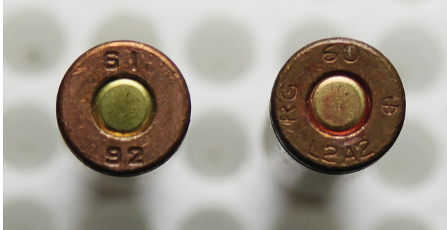
Figure 3.2 A study of two Chinese-sourced cartridge head stamps. On the left is a typical example of 7.62×51mm ammunition of Chinese origin using block characters. The 61 indicates the factory number; 92 indicates that this cartridge was manufactured in 1992. The example on the right, also 7.62×51mm, is a forgery. The head stamp indicates production by Royal Ordnance Radway Green in 1960, complete with NATO standard cross. L2A2 was the British military designation for the 7.62×51mm NATO ball cartridge. Both examples are of similar construction; the casing is copper-plated steel. (Image from author’s collection.)
